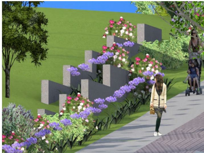
The rendering above shows an offset pair of stepped retaining walls to accommodate the significant grade change, interspersed with planting areas.
